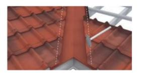
Purlins should be placed at **32 cm** centre tot centre. The distance between the first and second battens **should be 27 cm** instead of 32cm. The overhang has to be **max 5 cm**.
