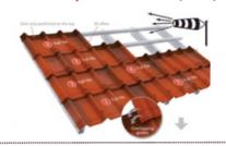
Cover the ridge line with the Standard ridge and fasten it on each side of the roof. Maximum distance from ridge point to next purlin is **15cm** and overlap between ridges
