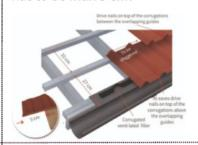
The aesthetics and wind upli protection can be optimized by using the verge element accessory, which is fixed first on the sidewall, then as well on the top of the corrugation.
